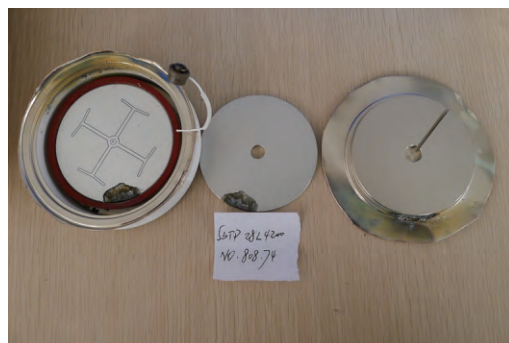
图 6 晶闸管过热击穿 Fig.6 Overheat breakdown of SCR
